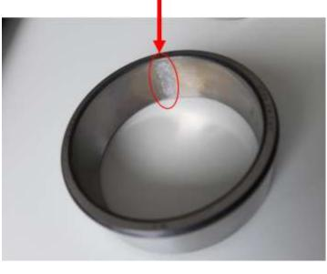
Characteristic damage frequency: Ball Pass Frequency of Outer race BPFO = f shaft \* BPOO BPOO = 4.724
